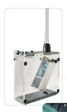
The Ball Impact Tester allows standardized impact tests for bottle closures. The bottle to be tested is held in a box, which can be swung from a horizontal to a vertical position in steps of 5 degrees.
