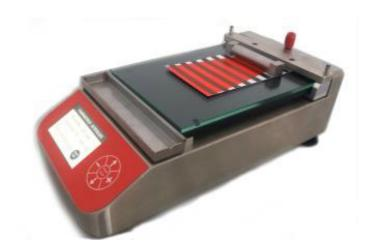
It obtains uniform and reproducible coating films/layers and works with a wide range of applicators. It is necessary if color formulation is required.
