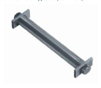
Film applicator of adjustable length Applicable to thickness in a range of 0 to 250 microns.. It can be adjusted making use of the markings on each side of the applicator. Produced in hardened stainless steel. Available width: 50 mm or 80 mm.
