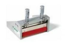
This film applicator includes two integrated micrometric screws to adjust the height of a knife. The distance of this knife can be adjusted in steps of 10 microns from 0 to 6 mm. Produced in hardened stainless steel.
