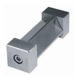
Film applicator with flat-edged prismatic body. Available in variable widths and at four different lengths: 50,100, 150 & 200 microns
