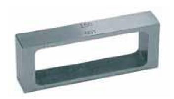
Multi-functional film applicator. Ideal for applying four different layer of thickness with a single equipment. Standard useful width of 60mm. Different sizes are available on demand. Produced in hardened stainless steel.
