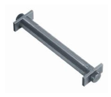
Film applicator of adjustable length Applicable to thickness in a range of 0 to 250 microns. It can be adjusted making use of the markings on each side of the applicator. Produced in hardened stainless steel.
