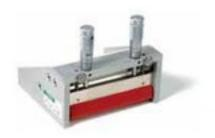
This film applicator includes two integrated micrometric screws to adjust the height of a knife. The distance of this knife can be adjusted in steps of 10 microns from 0 to 6 mm. Produced in hardened stainless steel. Available in 3 width3:100mm, 150mm and 200mm
