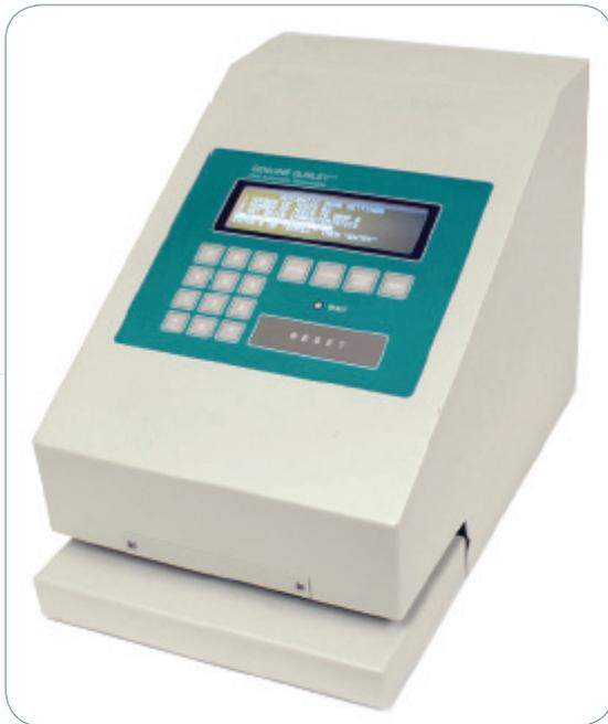
This unit measures the air permeability and smoothness of all kind of sheet materials. It combines the abilities of textile, standard and high pressure densometers, S-P-S testers as well as programmable digital timers.
