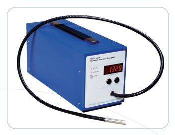
Our moisture content analyser is a non-contacting instrument for moisture measurements in real time.
