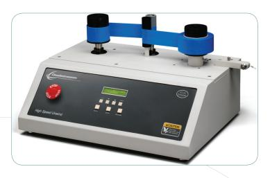
Accurately measure the unwind force of a roll of tape with the ChemInstruments High Speed Unwind Machine. The High Speed Unwind Machine meets the standards specified in ASTM D 1000 and AFERA 4008 for unwind force at a fast rate of removal. It will also test the unwind force of pressure sensitive tapes according to Test Methods PSTC-8 and PSTC-13.
